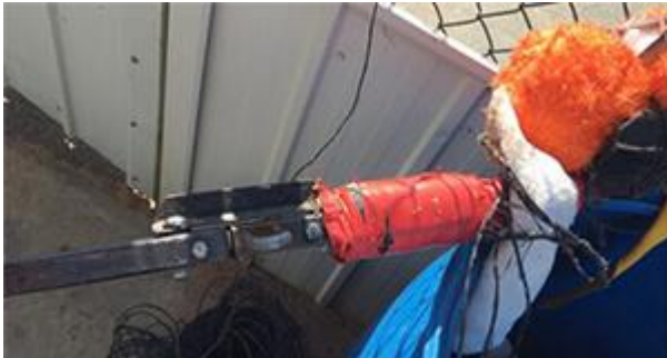
This lure is not acceptable because it has sharp edges that may injure the operator or the greyhound.
