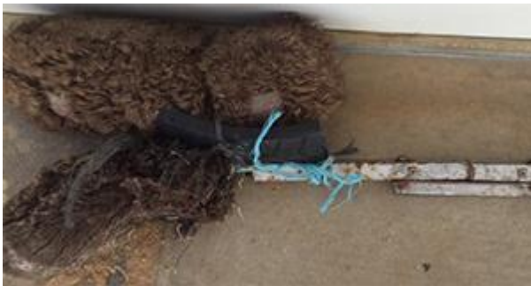
This lure is not acceptable because it has sharp edges that may injure the operator or the greyhound, and it is made of lamb's wool, which is an animal material.
